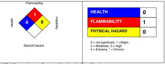
NFPA Flammable and Combustible Liquids Classification Combustible Liquid Class IIIB
